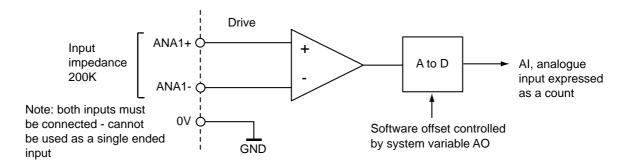
Figure 3-12. Analogue Differential Input
